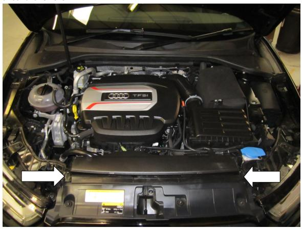
3. Using your T27 torx drive remove the three fasteners arrowed .
