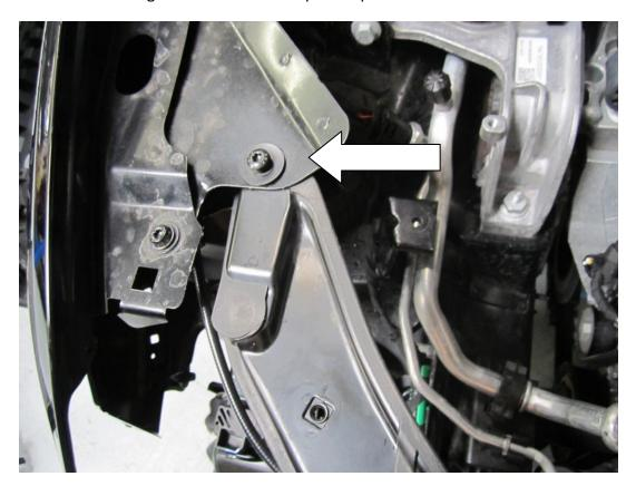
37. Place the condensor onto the intercooler brackets. In order to clamp the condensor to the intercooler without having to disconnect and regas your aircon, two small holes must be drilled in the plastic cowling. Mark a position inline with the clamps on your plastic cowling. Using a 5mm drill bit, drill the holes to allow access with an allen key to do up the clamps.
