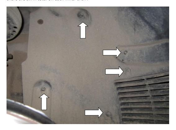
8. Pull back your arch liner then using your T25 torx drive remove the two fasteners pictured.
