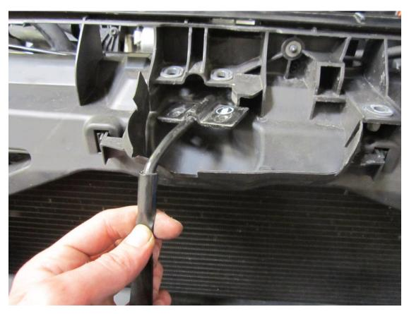
17. Disconnect the loom that connects to the bonnet latch sensor. This is located towards the middle of the plastic cowling beneath where the duct sat to the airbox.
