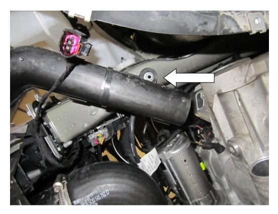
19. Disconnect the air temp sensor on the lower side of the crash bar
