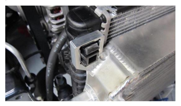
35. Place the new black plastic brackets on your intercooler to replace the old brackets. They only fit one way up. Two screws and washers are provided to hold these in postion. Keep the screws to hand to use shortly.
