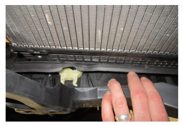
27. Using a flat bladed screwdriver, push the clips on the intercooler to release the condensor. This will need to be slid upwards while pushing the two upper clips.
