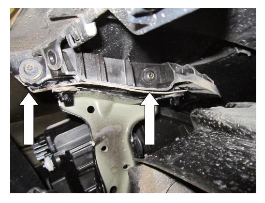
9. Again using your T25 torx drive remove the fastener that is located where the bumper meets the front of the inner wing. This is located beneath the headlight and can be accessed from the inner arch.
