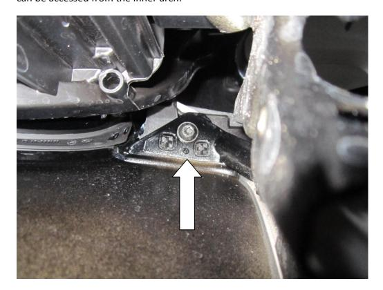
10. Located on the lower of the radiator cowling, disconnect the loom that controls the head light washers on the front bumper.
