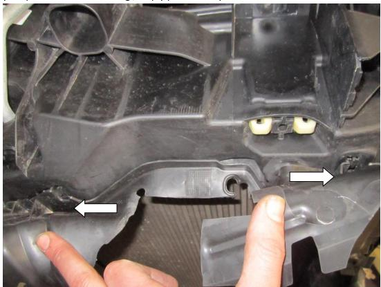
24. Now remove the large white brackets that hold the radiator pack into the cowling. These often break but dont worry, new brackets are supplied with your new intercooler.
