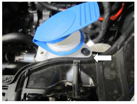
16. Using your T27 driver, remove the fasteners that hold the front crash bar lock bracket in place and remove.
