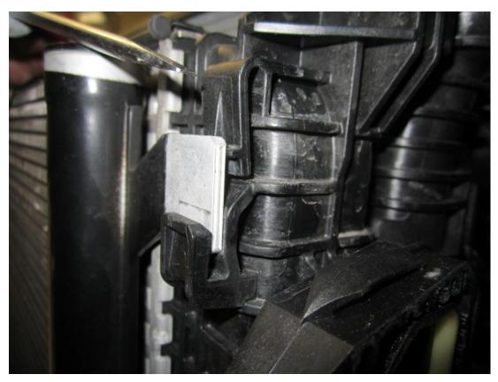
28. With the condensor loose pull the intercooler and radiator out of the plastic cowling. It is held in on two pins that locate in the bottom of the plastic radiator housing. This is easier with two people! Rest the radiator and intercooler on the jack and pull the cowling to one side. It cant be removed as the air con pipework threads through it. Take caution so as to not damage your air conditioning pipework to the condensor.
